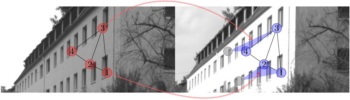
Figure 4.1: Illustration of the graph matching problem. A graph is constructed using annotated tracks in the reference image (left). We want to find assignments of the tracks in the target (right) such that the graph edges are most similar in reference and target frame. The arrows illustrate the assignment. The blue surfaces around the target tracks denote possible candidate sets  $PT_n$ . The grayish circles correspond to unrelated target tracks.
